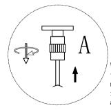
When adjusting the height of the steel wire, the telescopic metal part A toothed outer ring can only twist half a turn, and then pull it up to adjust the height!!! 2116D26 D26" H5. 11" L15
